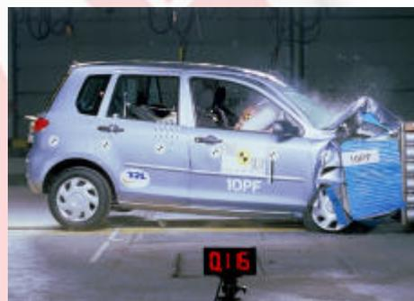
NCAP to encourage manufacturers to exceed these minimum requirements. The Euro NCAP tests include front impact, side impact, pole impact and pedestrian safety. Cars are given scores in each test and are then awarded an overall 'star' rating.
